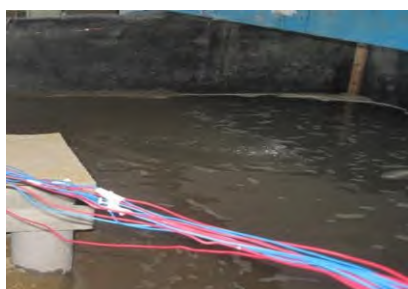
图 8 砂土完全液化 Fig.8 Complete liquefaction of sandy soil
